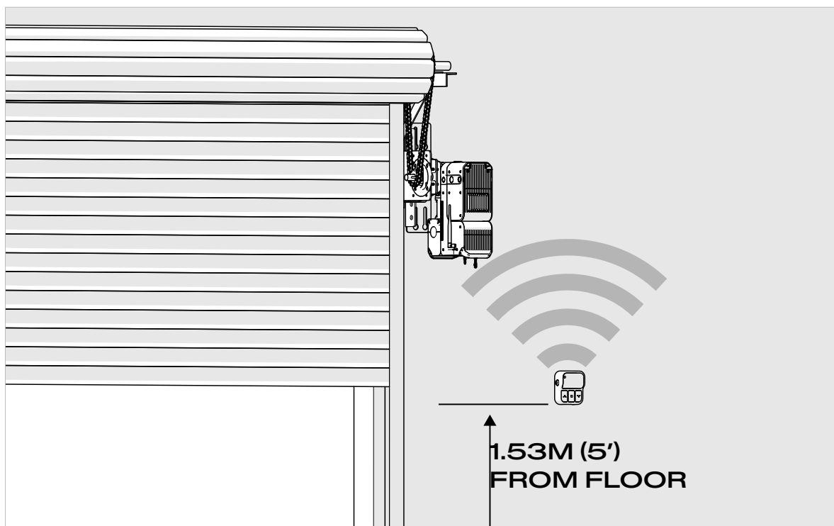
Typical setup with wireless console connection
